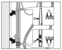
■ Secure the transit bars to the back of the washing machine. Make sure that holes (B) are fitted over retainers (A).
